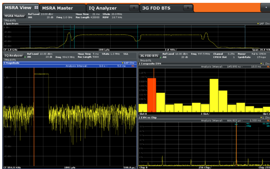
Figure 10-5: MSRA View of MSR signal with time correlations
