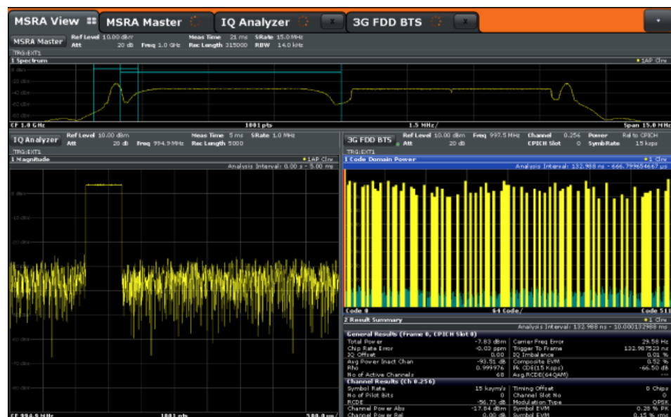
Figure 10-1: MSRA View for I/Q Analyzer and 3GPP FDD BTS slave applications
